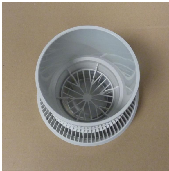
Figure 4 Internal view of STUDOR MAXI-VENT, KNITS II and OsmaVent 110
